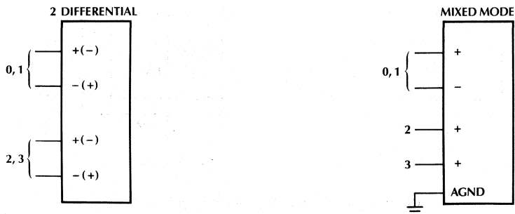
Figure 7. Analog Input Multiplexer Functional Options for ML2283
