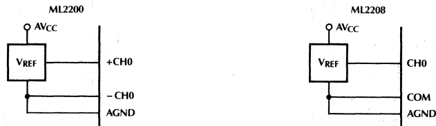
Figure 19. Using a 2.5V External Reference
