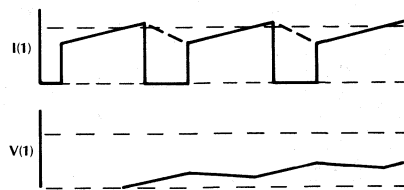
Figure 4. Switching Current and Pin 4 Voltage — Normal
